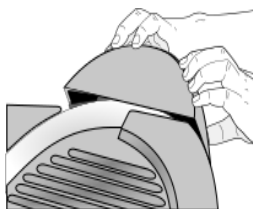
FIG 3. INSTALLING THE SHARPENER BOX
